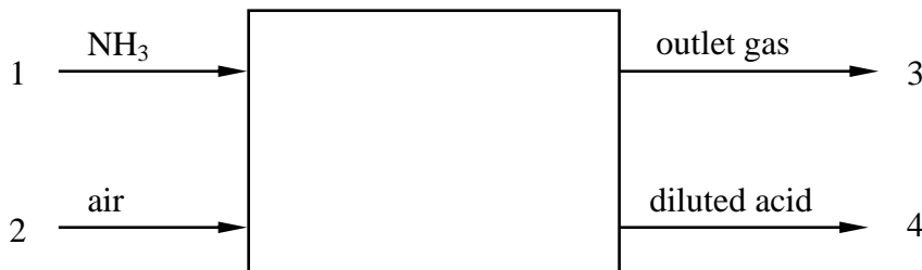
Fig. 3-2 Oxidation of ammonia
